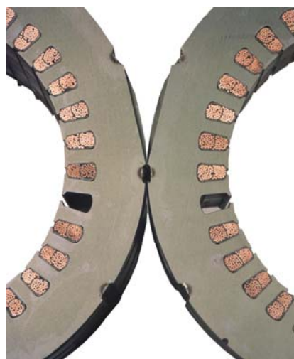
Stator section showing resin penetration
