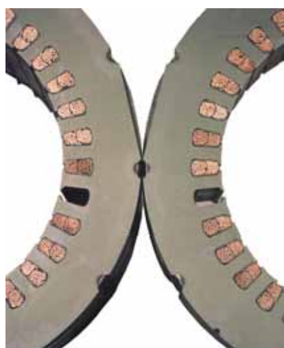
Stator section showing resin penetration
