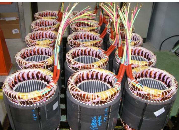
ELECTRIC MOTORS STATORS (PARTICULAR)
