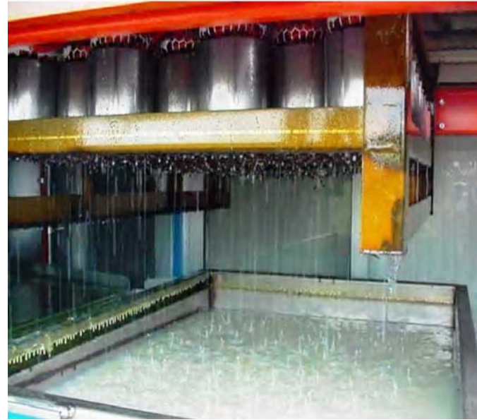
DRIPPING STAGE AFTER IMPREGNATION
