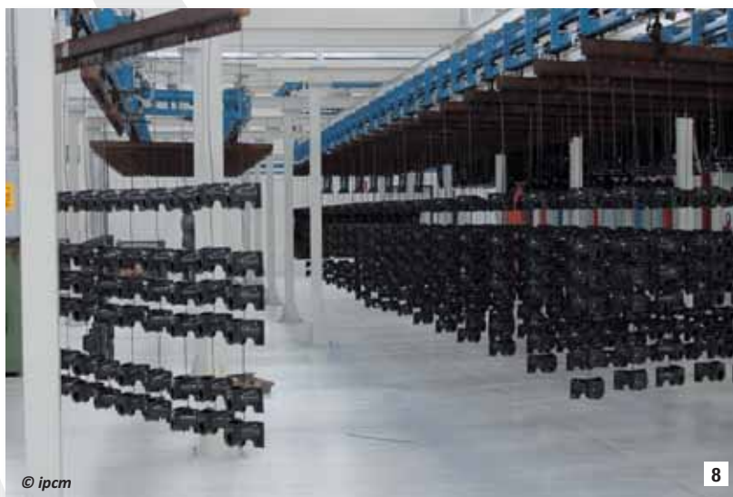
8 Storage buffers for the suspended tray conveyors. I polmoni di accumulo delle bilancelle.
