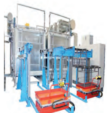
U-type dipping impregnation line
