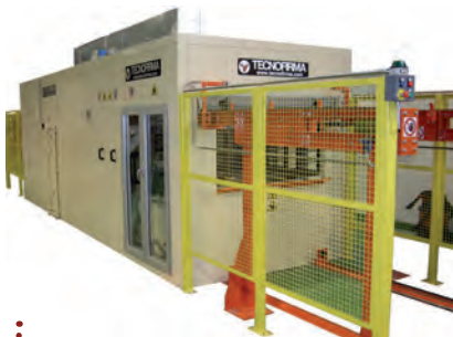
Cold dipping impregnation line
