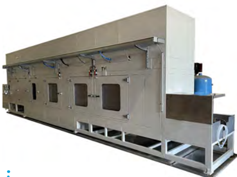
Tunnel with pallet chain conveyor for automotive components
