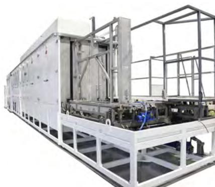
Tunnel with recirculating pallets for battery housing
