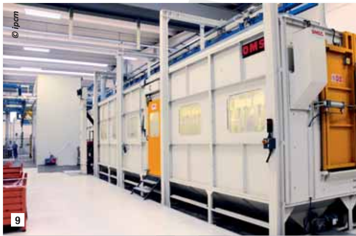
The shot blasting plant by OMSG La granigliatrice OMSG.
