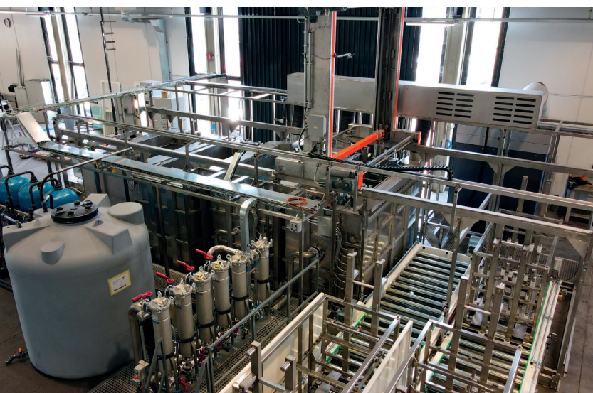
Multistage positioned washing machine for battery housings. Dip washing machine for battery housings.
