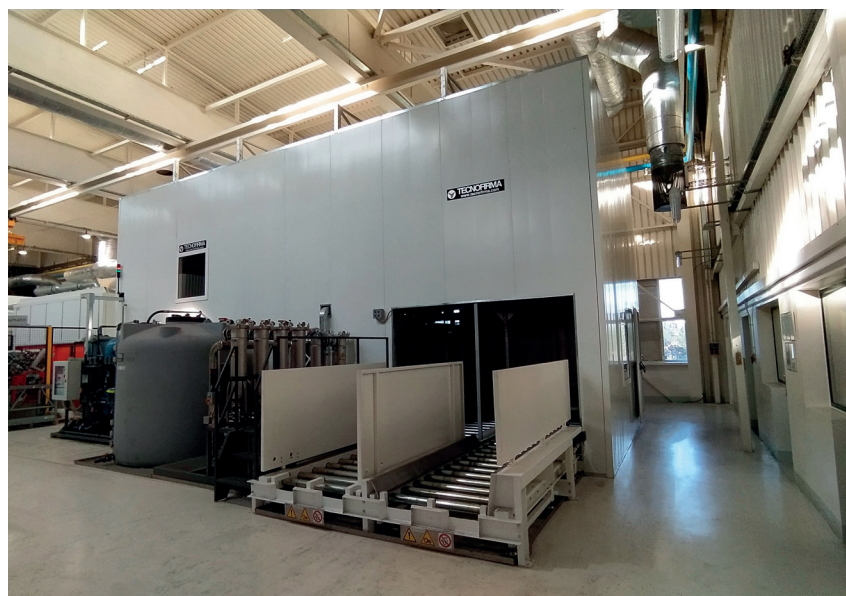
Sat-Lin washing machine for battery housings. Intermediate dip washing machine for battery housings.
