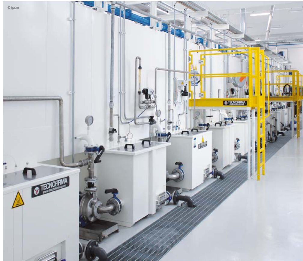
The 13-stage pre-treatment tunnel.
