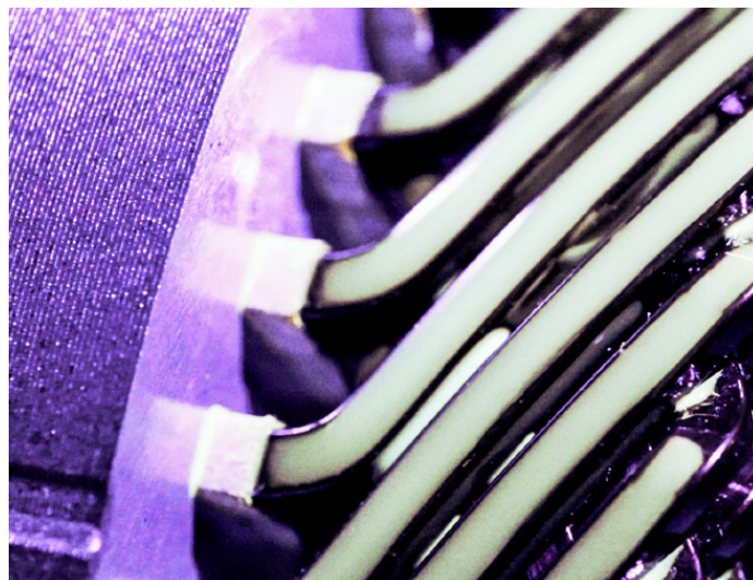
Hairpin stator with applied resin
