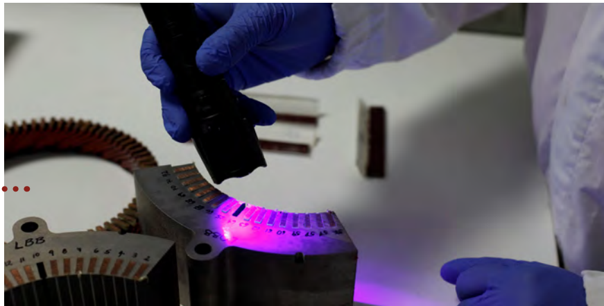
• Powder Coating for hairpin stator • Pulver-Beschichtung für Hair-Pin Statoren
