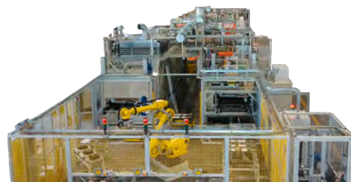
U Line equipment for hairpin impregnation high productions U-Line Anlage zum Serien-Produktion von Hairpin Statoren
