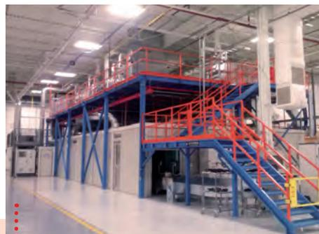
• • • **Hardcoating line for polycarbonate lenses of automotive headlights**
