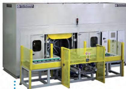
• Hydrokinetic washing plant for big parts
